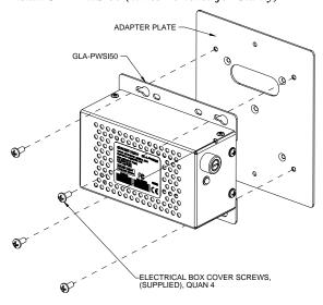
**NOTE:** The GLA-PWSI50 should never be installed with the label facing down.
